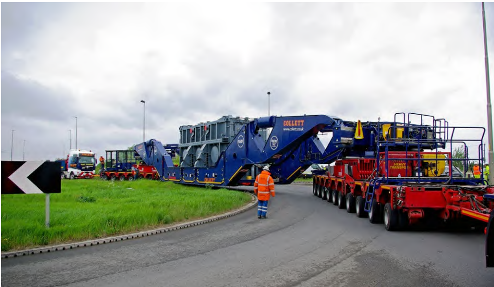
Image of large transformer being delivered to site on the abnormal indivisible load (AIL) vehicle.
